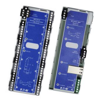
MTL830C-MBT analog multiplexer system with Modbus TCP® output provides a cost-effective alternative to single-loop isolation. The cost of installed wiring is reduced by up to 50% by communicating the input of multiple hazardous-area sensors over a single twisted pair data highway. Further savings are achieved by reducing the number of inputs to the host, cabinet space and weight.
